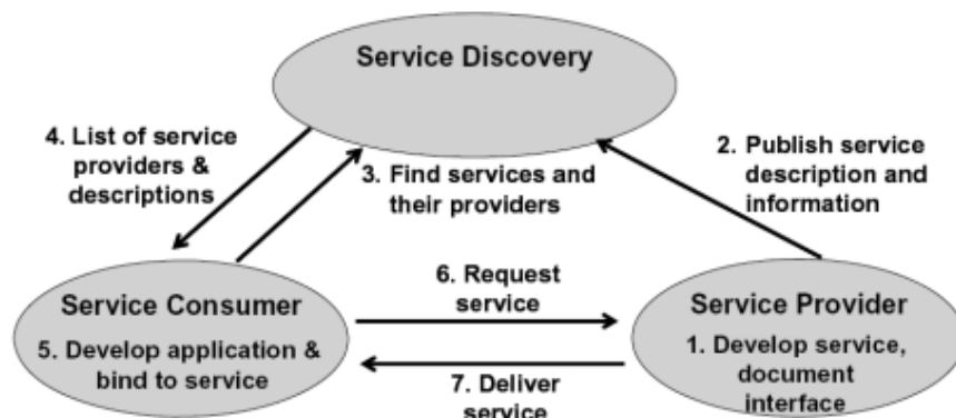
Fig. 1. Overview of roles in Service-Oriented Architecture (SOA). [4]
