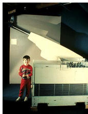
UNIMATE originally automated the manufacture of TV picture tubes
