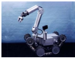
HAZBOT operating in atmospheres containing combustible gases
