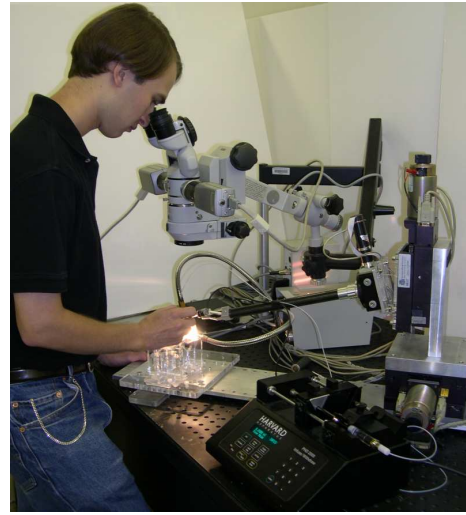
Fig. 7. The new steady-hand manipulator for retinal surgery during a CAM vein cannulation.
